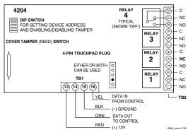
Figure 11. 4204 Connections to Control
